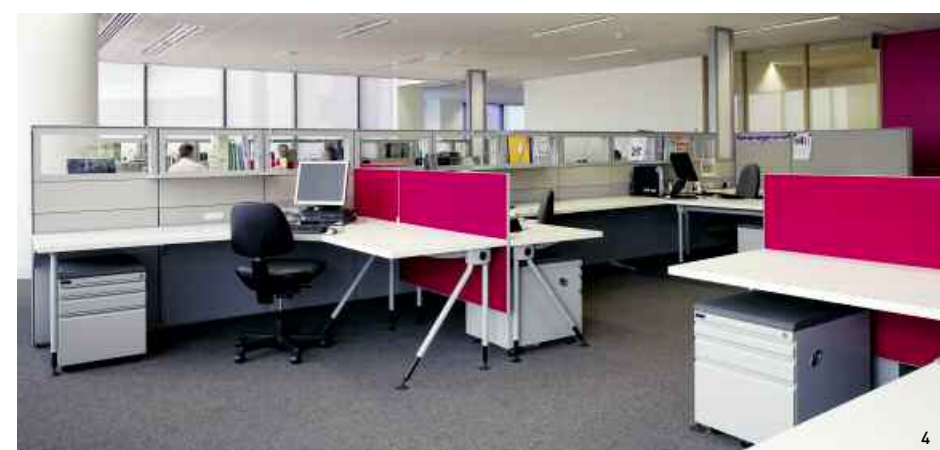
1_Level 27's lustrous reception area. 2_Unimet workstation screens with panel mounted worktops and QED returns, pedestals with fitted side-pull handles and cushion tops, desk clamped slimline panels, metal transom mounted shelving. 3+4_Workstations as per image 2, with passage screens featuring perforated metal tiles, powerblades with coloured Perspex.
